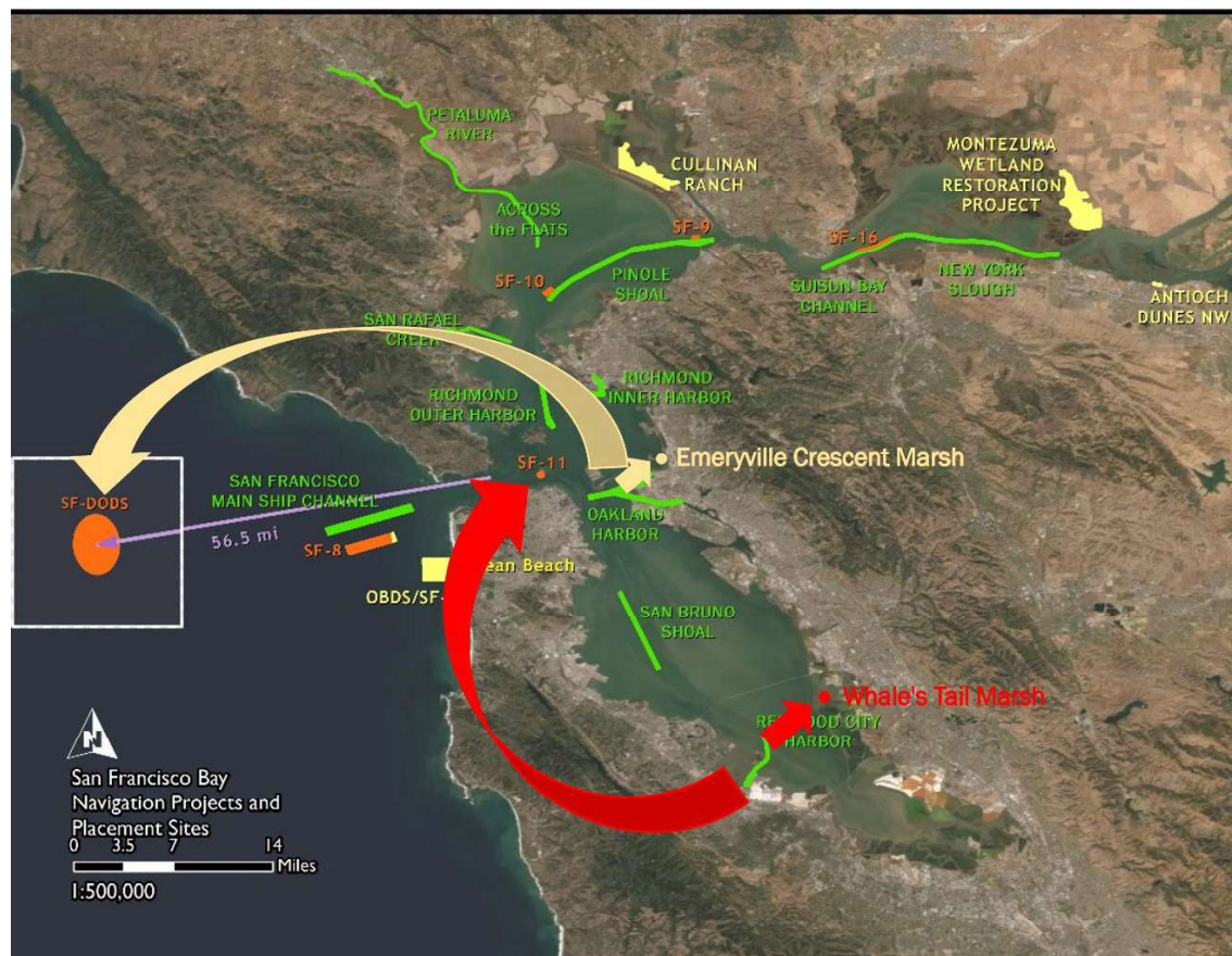
Figure 3-4. Transport pathways from the dredging projects linked to the two alternatives to their Federal Standard and Section 1122 disposal sites for the two alternatives. Red designates Alternative A (Whale's Tail Marsh), and yellow designates Alternative B (Emeryville Crescent Marsh).
